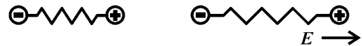
Figure 3.5 Atomic polarization results from the relative displacement of electrically charged ions on response to an electric field E .
